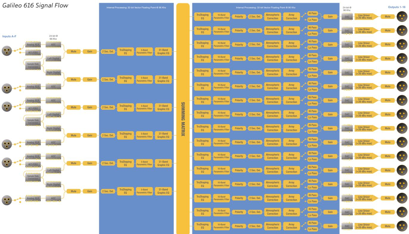
The Galileo 616 includes a powerful arsenal of DSP for tuning and aligning Meyer Sound loudspeaker systems. In addition to standard DSP components like delay (up to 2 seconds), gain, and polarity reversal, the Galileo 616 boasts an unprecedented architecture of equalization and filtering capable of addressing a range of acoustic anomalies and subjective tailoring of system responses, without introducing excessive shifts in phase that degrade intelligibility and signal clarity.
