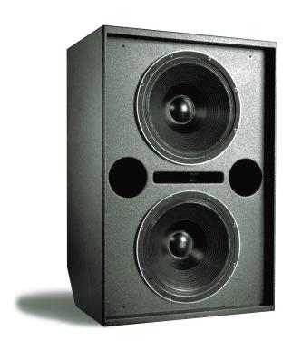
The 650-P is a self-powered, tuned, bass-reflex subwoofer that uses two 18" drivers, capable of long excursion with minimal distortion. The unit extends the lower range of Meyer Sound reinforcement systems by providing a frequency response of 28 to 120 Hz. Being self-powered, the amplifiers and control electronics are fully contained within the speaker enclosure.
